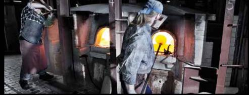
This mixture is placed in the furnace and smelted for 14 hours at 1450 degrees Celsius and prepared for the most important processing step, the glassblowing.
