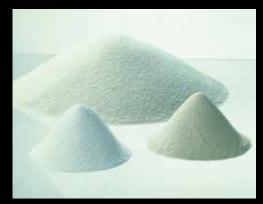
Quartz sand, soda and limestone constitute the basic mixture. The ratio of the three components varies depending on the type of glass. According to the required color, the various metal oxides are added.
