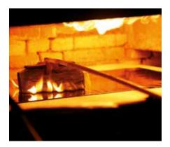
After cooling, the cylinder is cut open length-ways and then heated again, laid open and relaxed in a further processing stage. The wavy sheet is flattened with a special piece of wood.
