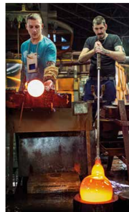
In a succession of wooden molds, the glass is given its correct form as it is simultaneously spun and blown.
