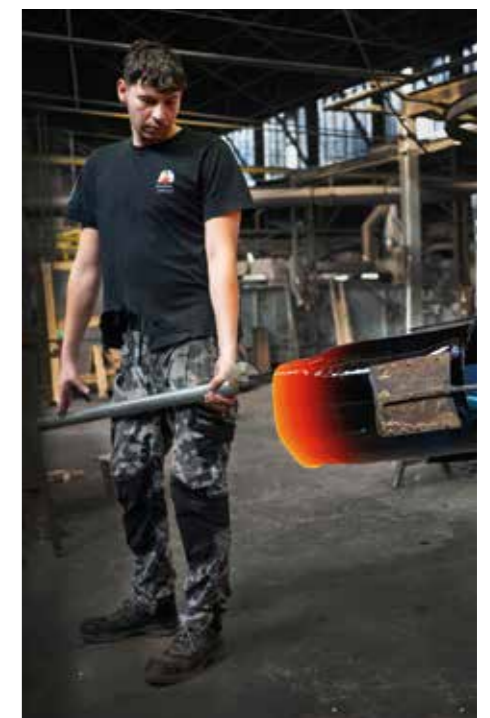
The glowing glass bubble is opened at both ends and widened, forming a cylinder.
