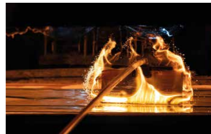
After cooling, the cylinder is scored with a glass cutter lengthwise and then heated again, laid open and relaxed in a further processing stage. The wavy sheet is flattened with a special block of wood.
