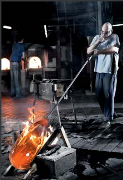
The simultaneous turning and blowing of the glass balloon produces the typical slight or more pronounced distortions in the glass surface.
