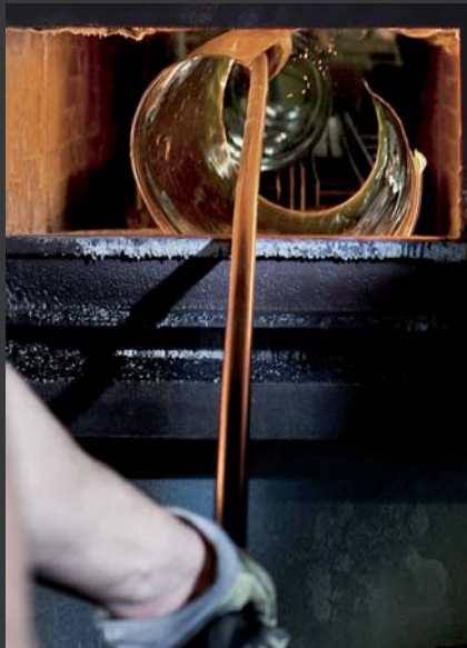
After being reheated, the cylinder is cut lengthwise, opened, and flattened.
