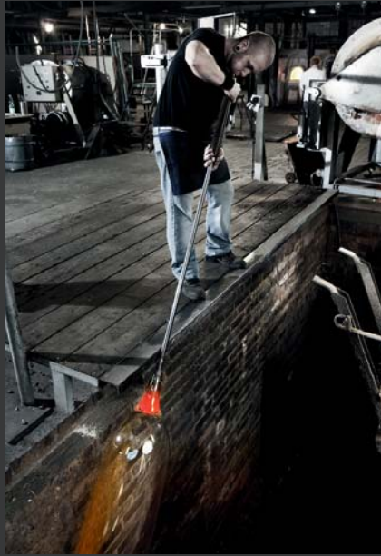
Production of restauro ® Light by swinging of the glass balloon in a deep pit, creates larger sheets exhibiting slighter distortions in the glass surface.
