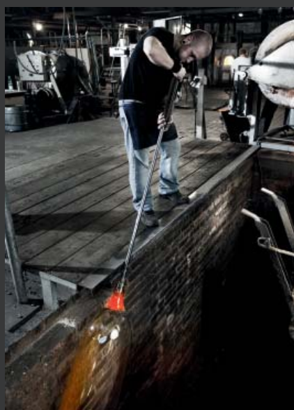
Production of restauro ® Light By additional swinging of the glass balloon in a deep pit, larger formats can be formed with slighter distortions in the glass surface.
