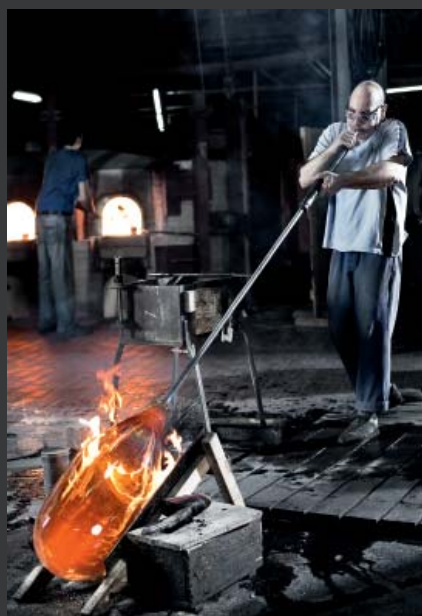
Production of restauro ® Classic The elongated glass balloon is formed by simultaneously turning and blowing.
